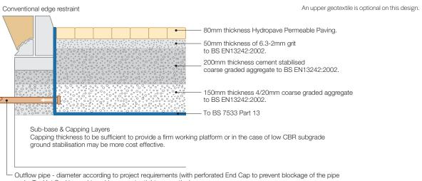
and a Top Hat Seal is used to achieve a water tight connection)
