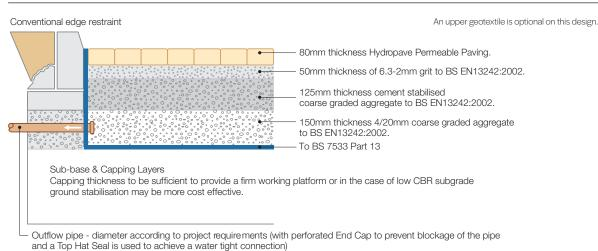
DBM (Dense Bitumen Macadam) can be used as an alternative to the cement stabilised coarse graded aggregate. Please refer to BS 7553 Part 13
