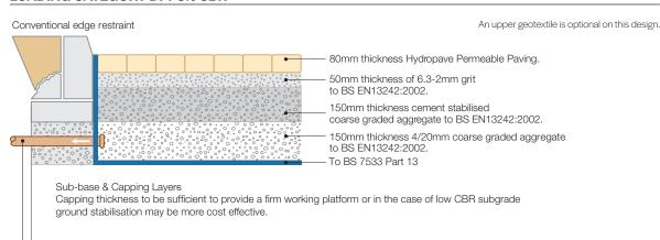
Outflow pipe - diameter according to project requirements (with perforated End Cap to prevent blockage of the pipe and a Top Hat Seal is used to achieve a water tight connection)
