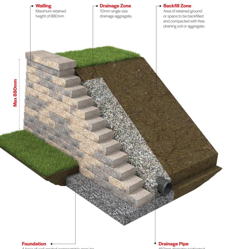
A base of well-graded compactable granular material or concrete alternative. One block remains below ground level.
