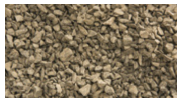
10mm single size drainage aggregate.
