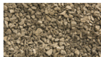
10mm single size drainage aggregate.
